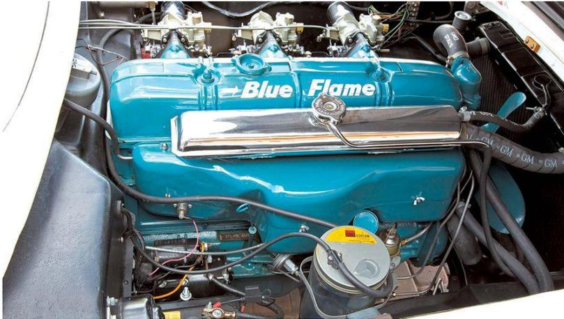
The Corvette legend was powered by V-8 engines, but it was an inline six-cylinder that started it all. Chevrolet's 235-cu.in. six was the only engine available in the Corvette for 1953 and '54. In '55, the 265 V-8 was offered as an option and most of the 700 Corvettes built were small-block powered, leading to the inline engine's demise in '56. More than 60
